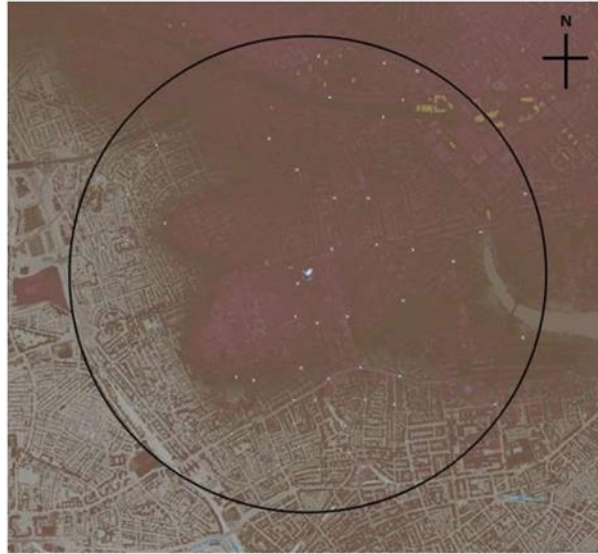
Figure 7-4: 50 Small Cell Base Stations Located within 1.69 km of Victim Earth Station in Central London
